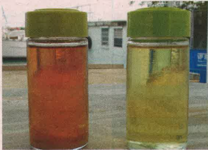
The before and after: the oil sample on the left is the raw product with which Marathon BioDiesel begins before he refines it to the sample on the right that efficiently and effectively fuels diesel engine vehicles.
